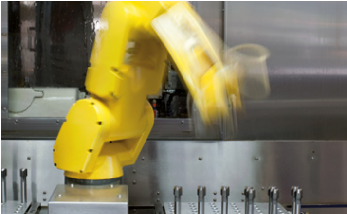
Robot-loaded grinding center
