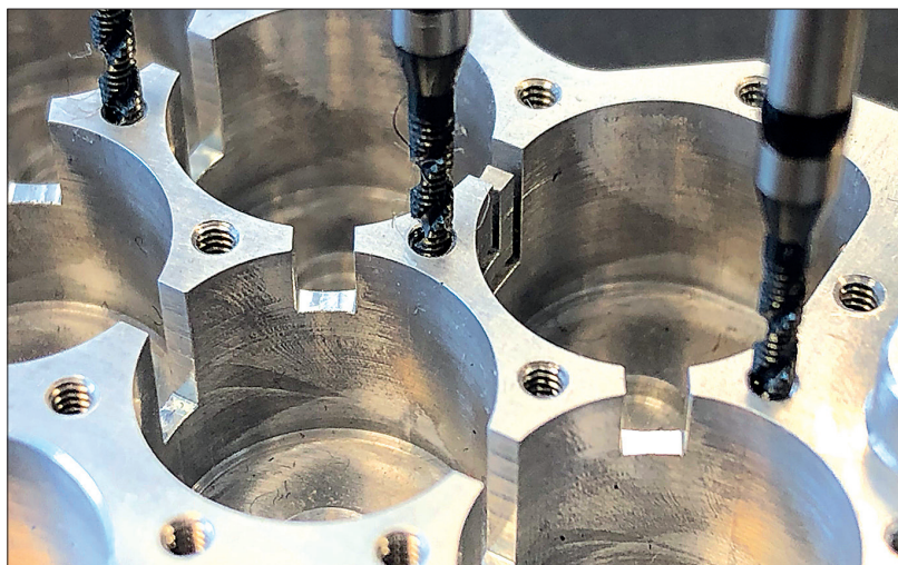
Aluminum space component with M1.4 threads
